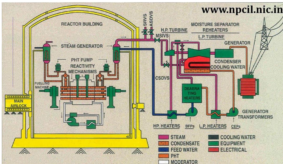
Figure 9: Schematic Representation of Pressurised Heavy Water Reactor (PHWR)
