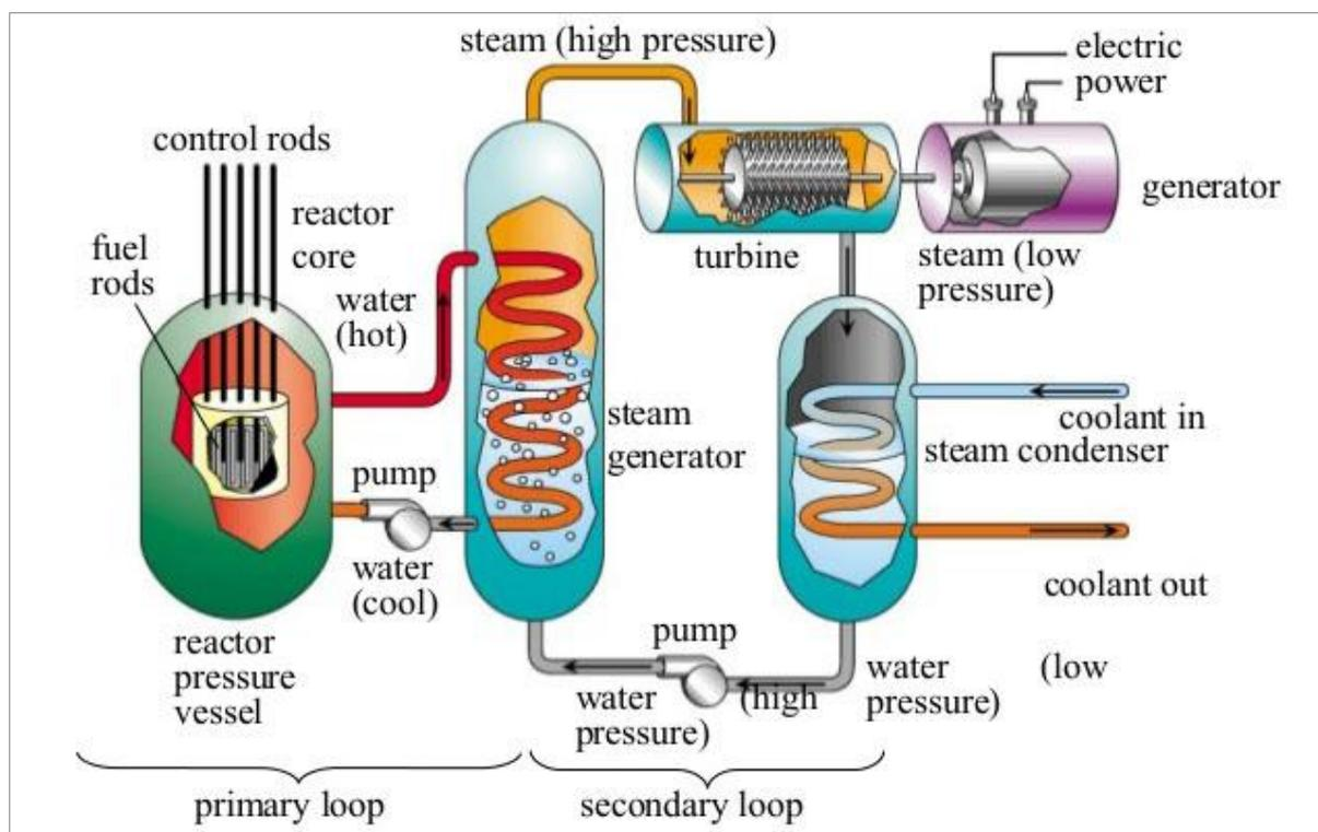
Figure 10: Schematic Representation of Pressurised Heavy Water Reactor (PWR)
