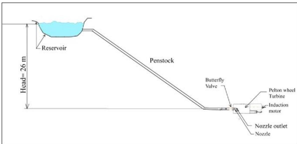
Figure 7: Schematic Representation of Micro Hydro Power Houses
