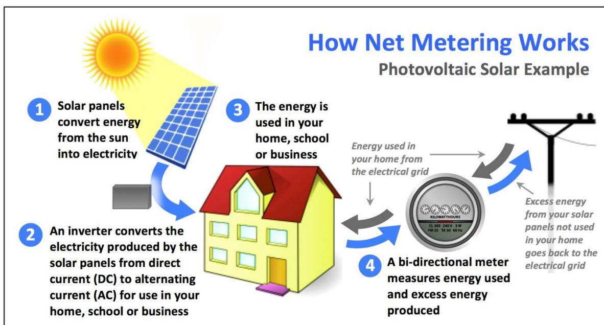
Figure 15: Solar Net Metering Concept
