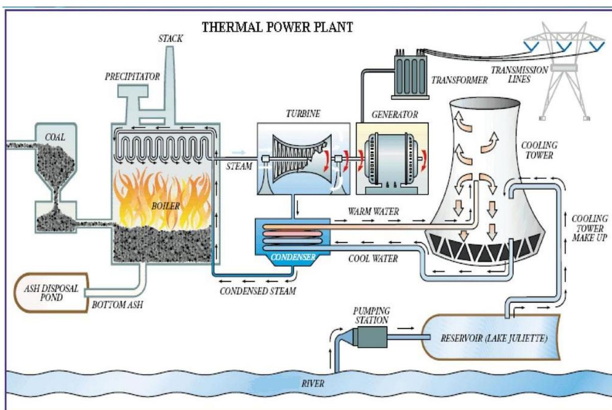
Figure 2: Process of Thermal Power Generation
