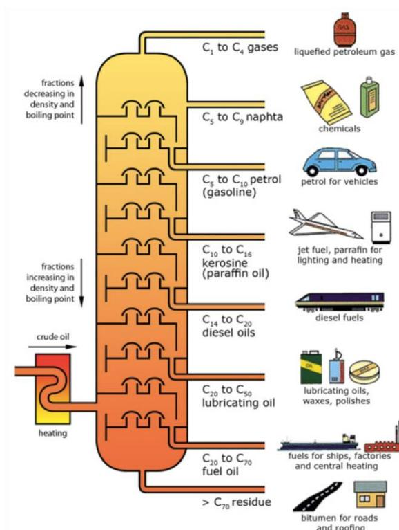
Figure 38: Fractional distillation of crude oil
