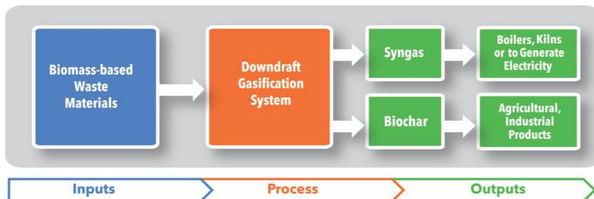
Figure 22: Process flow of Bio gasifier plant
