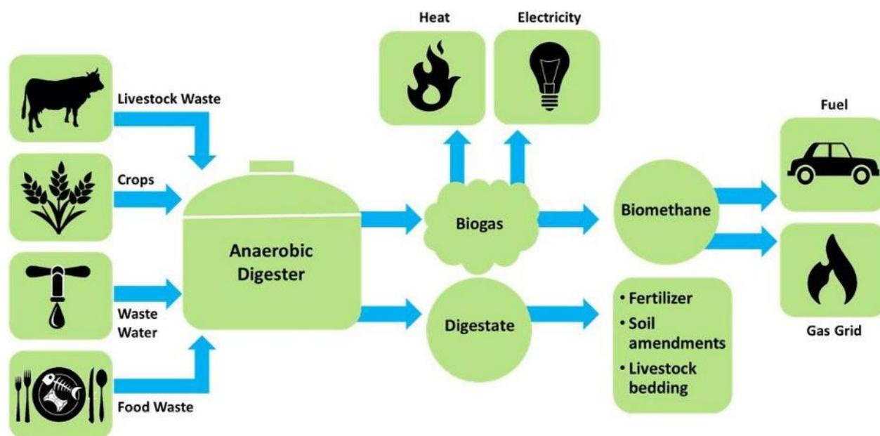
Figure 23: Process flow of Biomethanation plant
